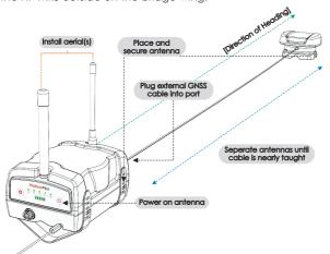
Within 2 minutes your LED's will be solid green when connected to your display. The Corrections LED will was be off if corrections are not available.
