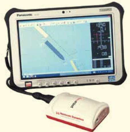
GyroPilot™ is the latest product in the Navicom Dynamics inventory, designed to provide a compact, lightweight, wireless source of comprehensive navigation data to a pilot's electronic charting system (ECS) when there is no requirement for the data to be independent of the ship's sensors.
